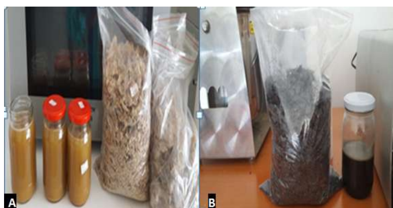
Figure 2: One kilogram of P. Amygdalus got 60% of oil as shown in A, N. sativa got 17% of oil as in B.
